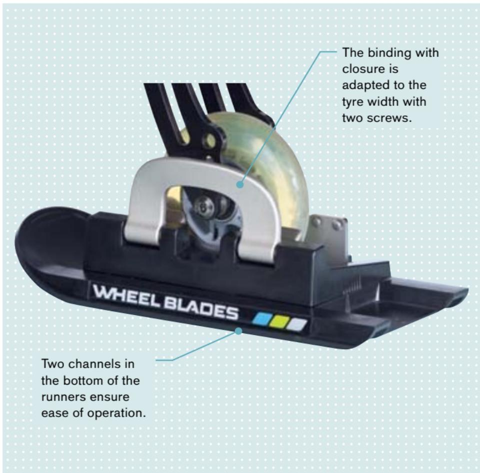
Thanks to optimum pressure distribution on snow by the runners, the wheels cannot sink in. Since the friction is very low, the runners are also able to compensate for larger surface irregularities.
