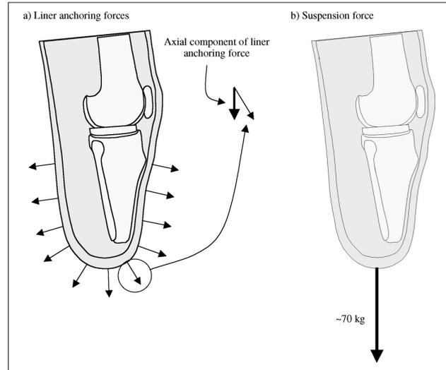
**Fig. 2** The vacuum creates forces that: a) anchor the liner to the socket. The sum of all the axial components of the axial forces creates a large: b) suspension force of ~70 kg. The suspension force prevents the liner/limb from extracting out of the socket.
