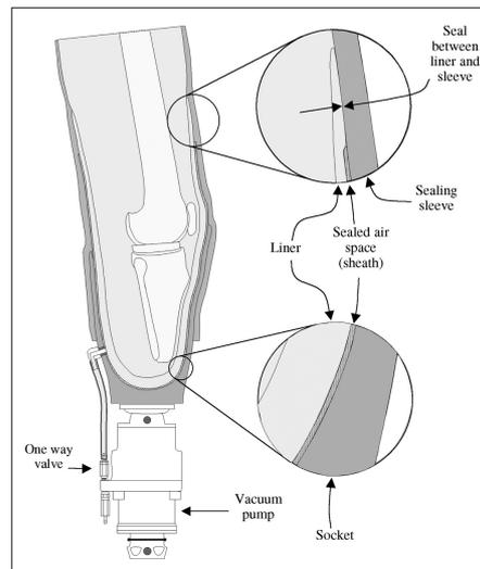
**Fig. 1** Cross section of vacuum suspension system showing sealed air space (sheath). Note that the sealed air space does not extend to the thigh. The seal between the top of the liner and sealing sleeve isolates the limb from the vacuum.
